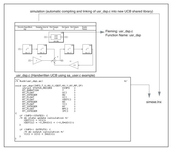
Figure 2-3. Linking Handwritten UCBs with the SystemBuild Simulator
